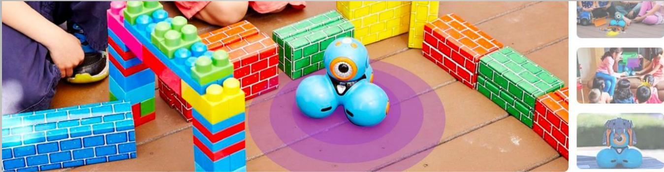
Front and back distance sensors allow Dash to detect objects and avoid walls.
